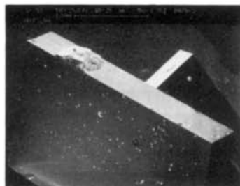
Fig. 2. YBCO crystals with major \{001\} and minor \{100\} and \{h0l\} faces (S 89).
