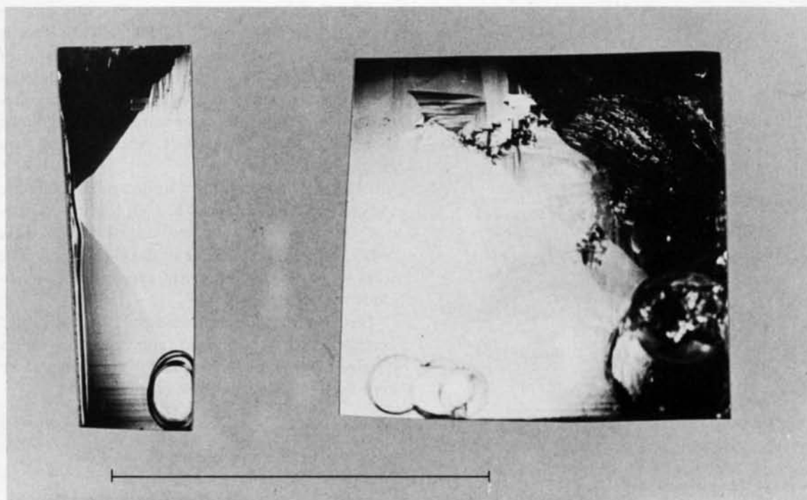
Fig. 9. KTa_{1-x}Nb_xO_3 crystal grown by slow cooling of the melt. The data of the actual growth experiment are given in table 3 (see No. 45). Marker represents 25 mm.
